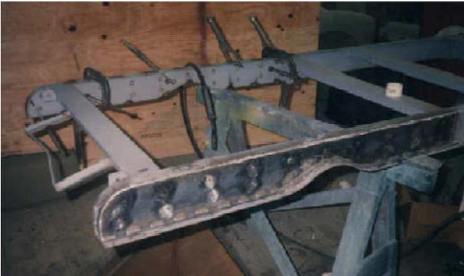
The aim of the modification is to strengthen the chassis in the vertical direction underneath the wheel indentation with another sheet of 1/8<sup>th</sup> inch steel so that it will not bend in the future.
