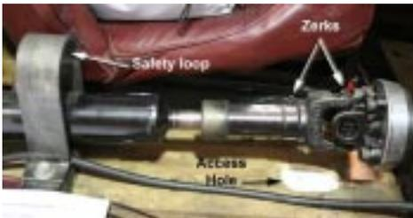
The new prop shaft with steel safety loop and access hole for zerks
