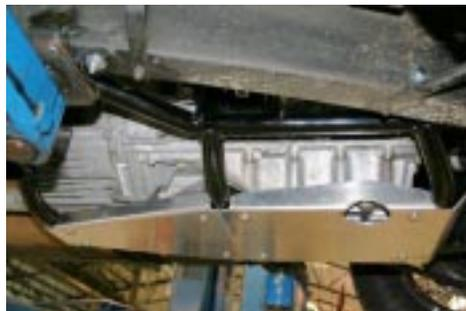
The motor mounts and skid plates from the side
