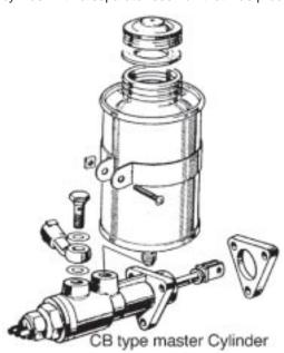
and know as a "CB" (compression barrel) master cylinder. Girling choose to produce at this time a cast steel (yes there is a difference between cast iron and cast steel) master cylinder without an integral reservoir. This may have been because it was hard or maybe cost
