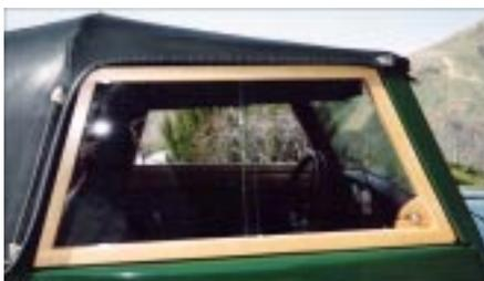
and angles on each end. With these cut I dry fitted the pieces for each window to make sure the joints were tight. Next I dadoed the grooves on the inside of the pieces for the windows: two each top
