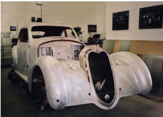
Undergoing total restoration at RX is a 1938 Alfa Romeo 8C 2900, owned by someone in Florida who picked RX for the restoration work. Powered by a 2900cc dual-overhead-cam straight eight with twin superchargers, this car, found several years ago in a Buenos Aires junkyard, in its day was the fastest production car in the world. The car won the famed 1947 Mille Miglia road race. It was restored once, but not correctly, and the Florida owner picked RX to do it right.
