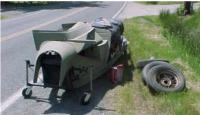
which was by now beginning to look a little more like a car, and then continued with work on the body. Making the body fit so all the spaces were equal was tedious work - more art than science. We hung, spaced, then rehung the doors; mounted the bonnet; put spacers between the wood frame and the chassis - you name it, we did it - until eventually all fitted really well and we were ready to send the body parts to the painter for painting.
